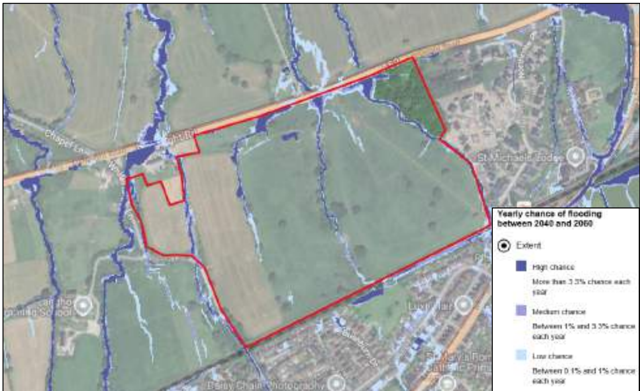
Figure 3: Environment Agency – Risk of surface water flooding map (2040-2060s, climate change scenario)
