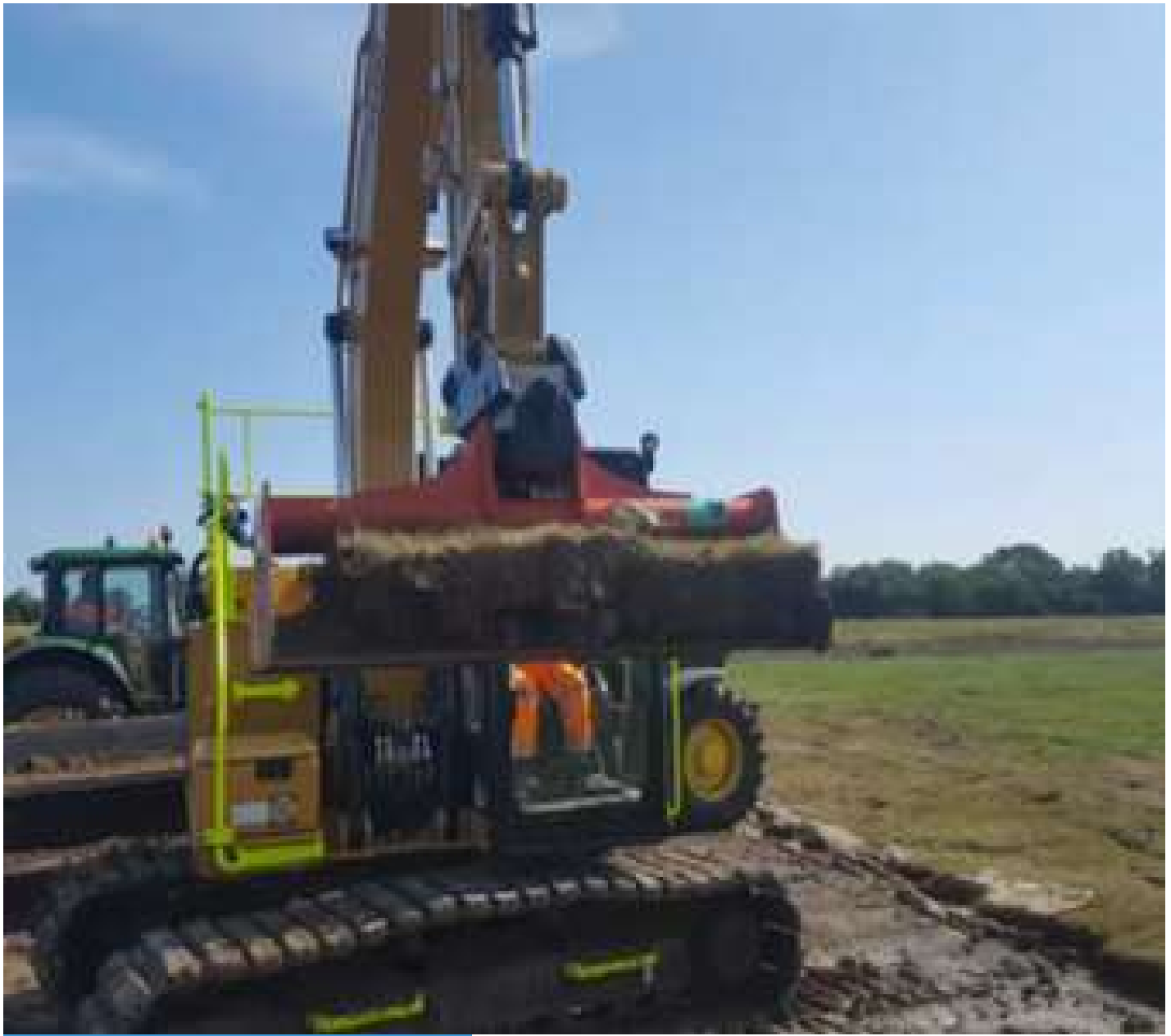
Figure 2c: Modified turf cutter used for taking turves from the trailer and placing at the receptor site.
