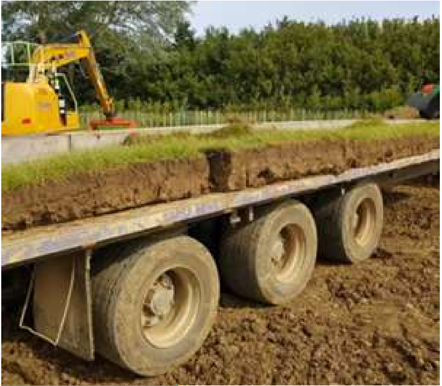
Figure 2a; Modified trailer holding turfs; central spine of trailer visible behind turves.
