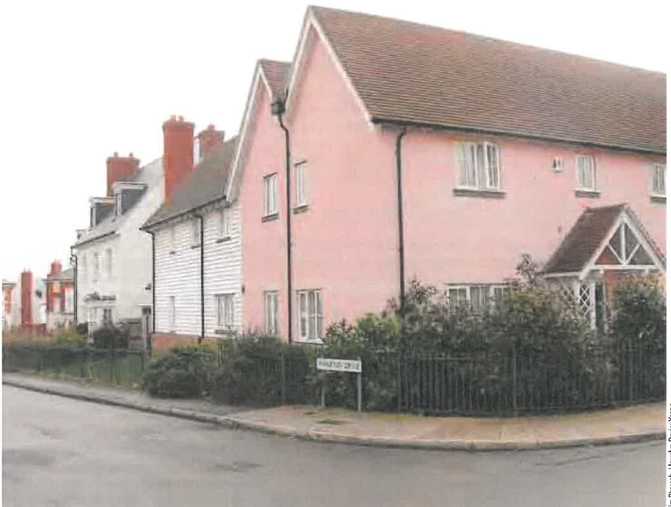
Figure 4.10 Active frontage to all streets and to neighbouring open space should be an aim in all developments. Blank walls can be avoided, even on the return at junctions, with specially designed house types.
