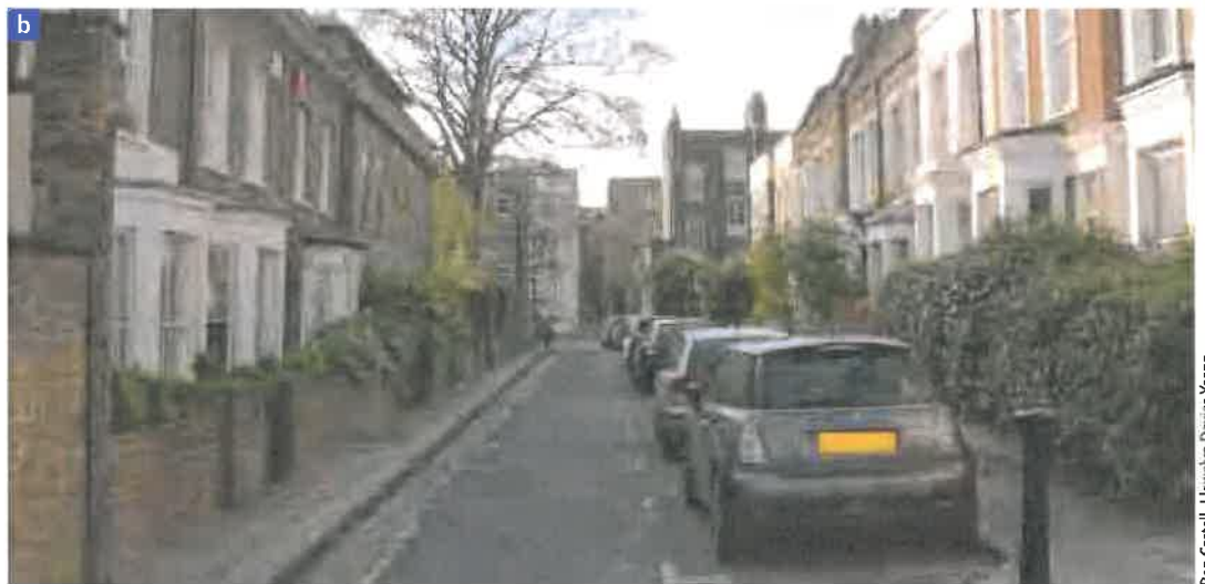
Figure 5.5 Two streets demonstrating different levels of enclosure. Street (a) has a height-to-width ratio of approximately 1:3, enabling a pleasant living environment to be shared with functionality in the form of traffic movement and on-street parking, some of it angled. Street (b) has a height-to-width ratio of about 1:1.5. Again, this works well in urban design terms, but the need to accommodate on-street parking has meant that traffic is restricted to one-way movement.
